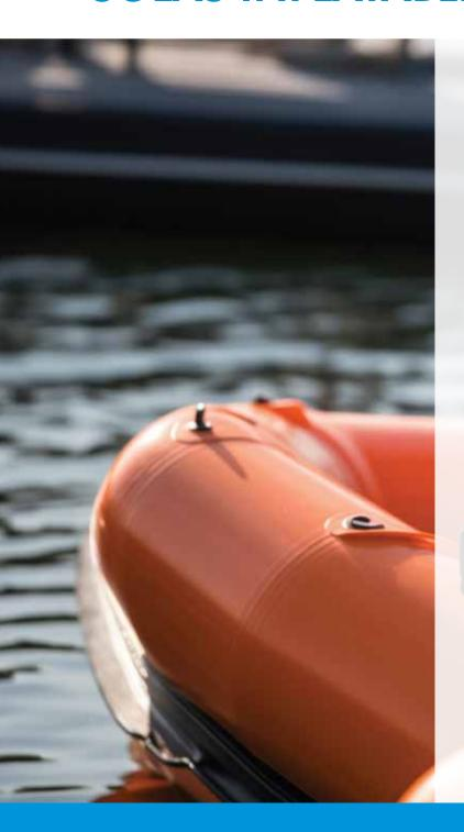
Inflatable Rescue Boat with EC/MED certification. Designed for maritime rescue applications as per the SOLAS convention, LSA Code 96. It meets the industry's highest safety regulations and is tested as per IMO MSC Resolution 81 (70).
